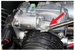
**Step 4:** Using a large flat head screwdriver pry the plastic charge pipe from the throttle valve. Only apply light pressure. (Image 4)
