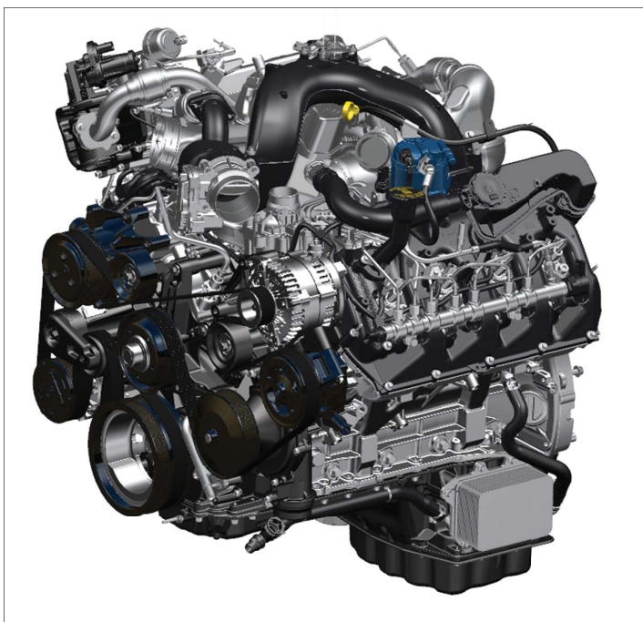
Secondary fuel filter location
