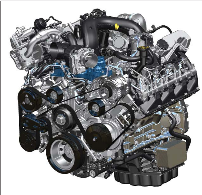
Primary thermostat location
