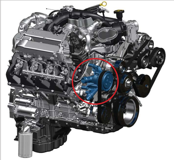
Secondary coolant pump location
